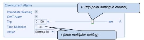
These settings provide for normal running of the generator up to 100% full load. If full load is surpassed, the *Immediate Warning* alarm is triggered and the set continues to run.
