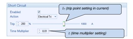
The effect of a short circuit on the generator is that the alternator stator and rotor begin to overheat; the aim of the *IDMT alarm* is to prevent the stator and rotor being overload (heated) too much. The amount of time that the alternator is safely overloaded is governed by how high the short circuit condition is.
