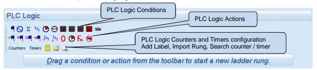
In PLC logic, the *ladder* of logic is made up of a series of *rungs*.
