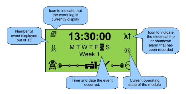
The events shown in the below table are recorded into the module's event log in addition to all electrical trip and shutdown alarms.
