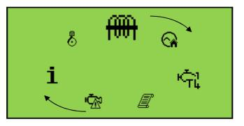
Once the desired icon is at the top, press the **Auto Mode**  $(\checkmark)$  button to enter that instrummentation section. If the **Auto Mode**  $(\checkmark)$  button is not pressed, the display automatically returns to the Home  $(\checkmark)$  page after the configured setting of the *LCD Scroll Timer*.
